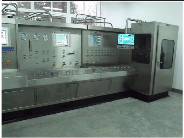
The integrated test bench for oil pump and accessories can test the oil pump and accessories assembled by aero-engine, including oil heat ex-changer, oil filter, etc., and provide different test solutions for research and maintenance units.
